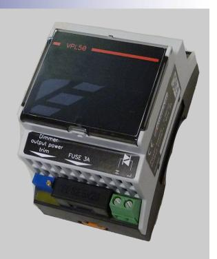
The VPL50 is a compact autonomous unit allows a power control of resistive or inductive loads with the phase angle modulated output. Designed for lighting or speed control on small single phase AC motor.
