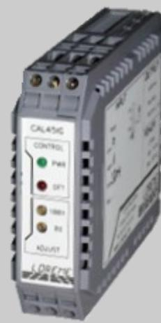
The CAL45 conditioner allows, for a Pt100, Tc, mA, mV or potentiometer input measure, to provide an isolated output current (4-20 mA). Their use is recommended for eliminating ground loops, or for the protection of the acquisition system.
