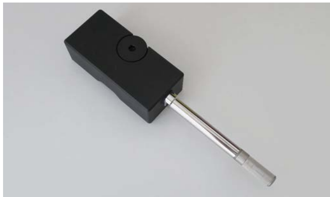
907037/1 probe shown with a stainless steel netting filter
