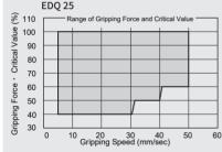
According to the intersection of 70% of the gripping force and 30mm/sec of the gripping speed, the latter is thereby judged to meet the requirement.
