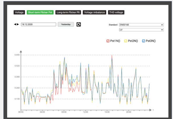
Progression of short-time flicker Pst during a day via the device website
