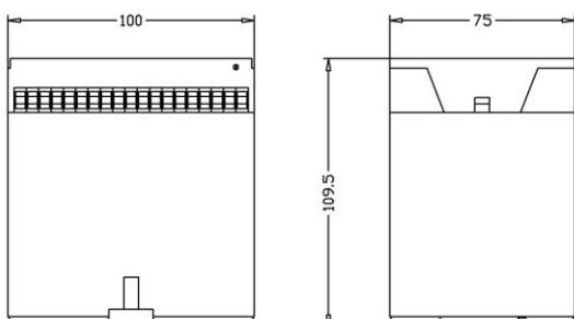
montaggio su profilo DIN EN 60715 TH 35 / DIN EN 60715 TH 35 rail mounting
