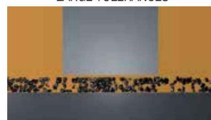
CONTAMINATION IN PRESENCE OF LARGE TOLERANCES
