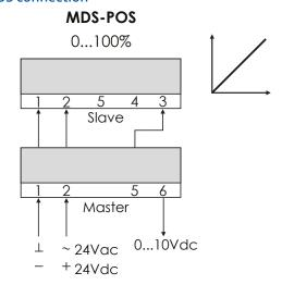
Parallel connection of maximum five MDS actuators is possible. The power consumption must be observed.
